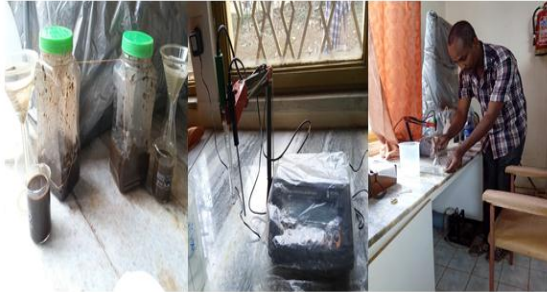
Figure 8: pH test by using HI2223 Calibration
