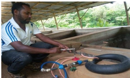
Figure 14: Bio gas burn test using Bunsen burner
