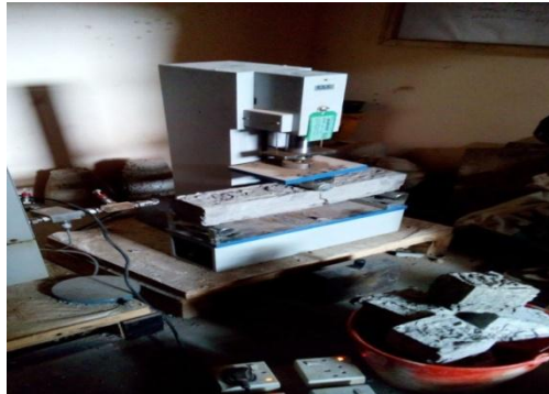
Plate 2. Flexural strength test set-up
