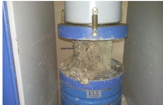
Plate 1 Compressive strength test
