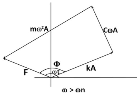
**Figure 3 Vector diagram for forced vibration with varying frequency ratio (a).  $\omega < \omega_n$ , (b).  $\omega = \omega_n$ , (c).  $\omega > \omega_n$**
