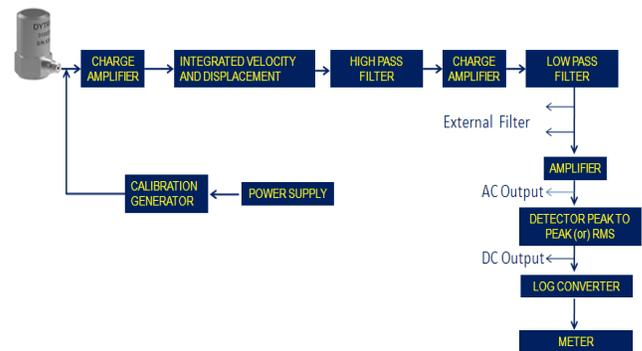
**Figure 9 Block diagram of measurement unit**
