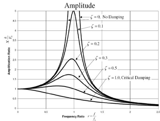
**Figure 6** Amplitude variations with respect to frequency ratio for various damping ratio
