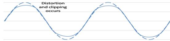
**Figure 11 Example of output distortions and clipping when supply voltage is low**
