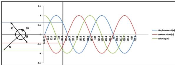
**Figure 2 Phase representation of displacement, velocity and acceleration.**
