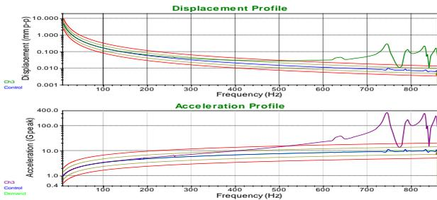
**Figure 12 Displacement (mm peak to peak) and acceleration (G peak) variation with respect to frequency (Hz), the red mark indicates an error produced in the reference channel**
