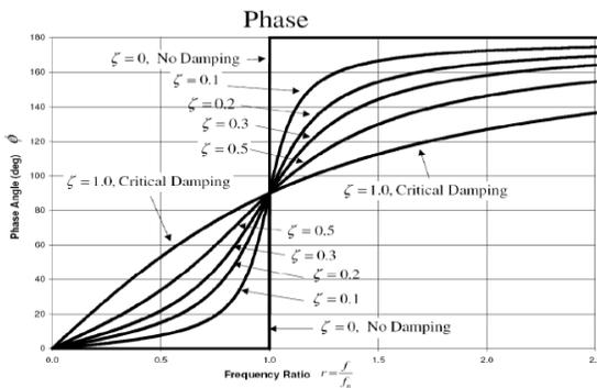
**Figure 5** Phase angle variation with respect to frequency ratio for various damping ratios
