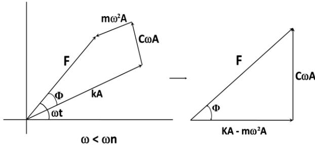
**Figure 4** The diagram shows that the applied force (F) is at angle  $\Phi$  relative to displacement (x).
