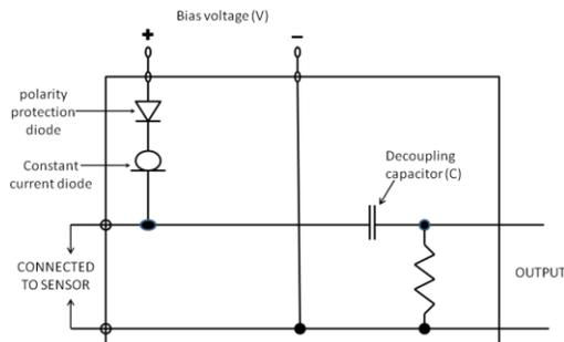
**Figure 10 Power supply of accelerometer**
