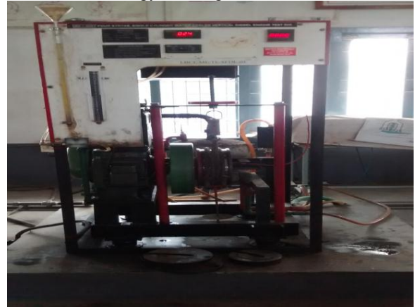
Fig: 4 Experimental Setup of Four Stroke, Single Cylinder, water cooled Diesel Engine.
