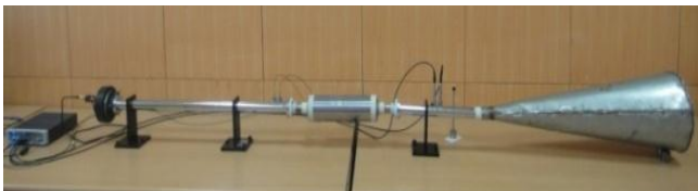
Fig 6 Impedance tube setup with anechoic cone in normal room facility
