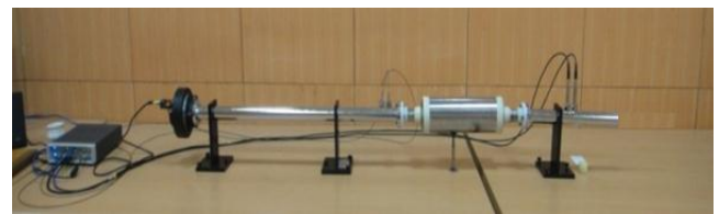
Fig 4 Impedance tube setup with anechoic sponge
