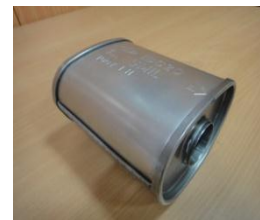
Fig 19 Absorptive resonator (muffler)
