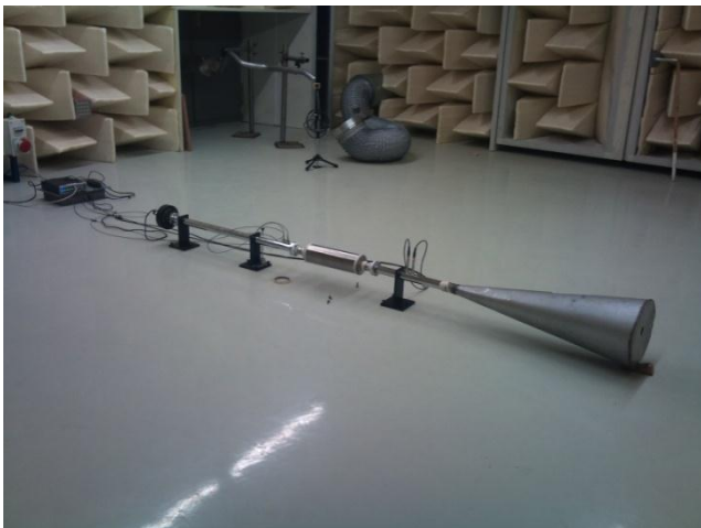
Fig 10 STL Test setup on anechoic lab with anechoic cone
