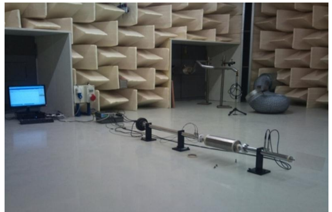
Fig 8 STL Test setup in anechoic lab with anechoic sponge
