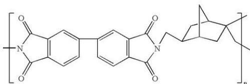
**Fig. 1: The structural formula of the novel isomeric polyimide**
