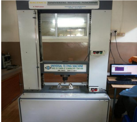
Fig 4.1: Electronic Universal Testing Machine interfaced with computer
