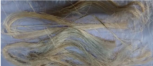
Fig – 3.2 Hybrid (sisal+ banana) fiber extraction
