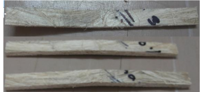
Fig6.1: Bending test specimen after testing
