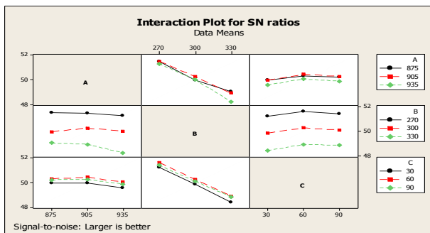
Figure 2 Interaction Plot (i) Austenitized temp Vs Austempered temp (ii) Austenitized temp Vs Quenched time and (iii) Austempered temp Vs Quenched time
