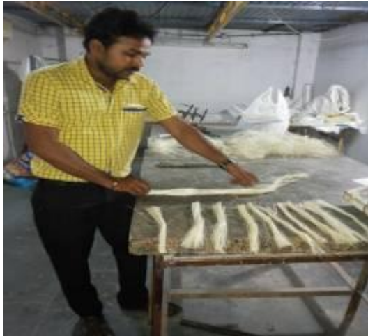
Fig -2. 6 Fiber Cutting for required length
