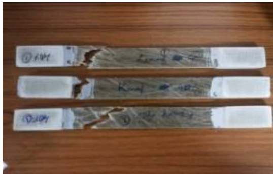
Fig4.1: Tensile test specimen after testing
