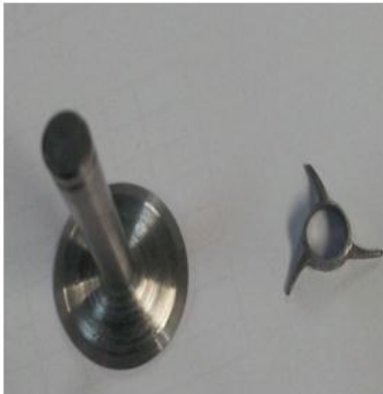
FIG-11 VALVE WITH 3 FINS
