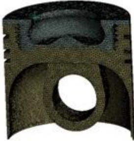
Fig 2: Meshed Sectional view of Modified Piston.
