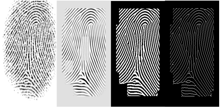
Figure 3: (a) Original Image, (b) Enhanced Image, (c) Binarised Image, (d) Thinned Image
