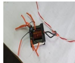
Fig 2.5 ETD Core Transformer
