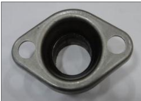
Fig 9 Sheet metal flange
