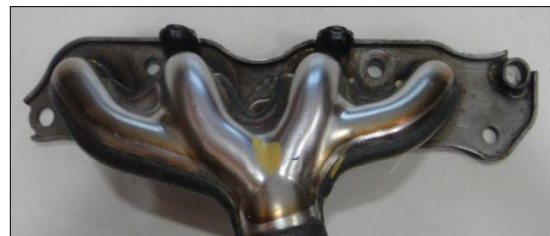
Fig 3 Sheet metal manifold
