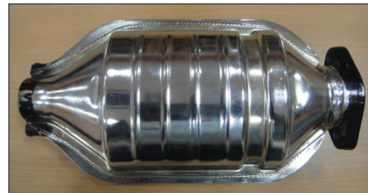
Fig 4 Catalytic converter assembly
