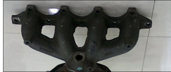
Fig 2 Cast iron manifold
