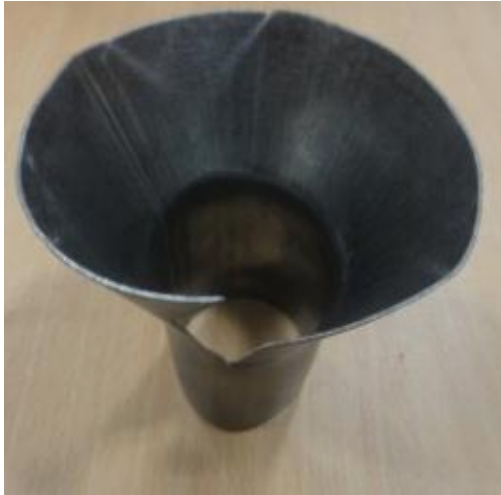
Figure 15 Crack initiated in base material
