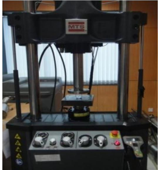
Figure 20 Flattening test Setup
