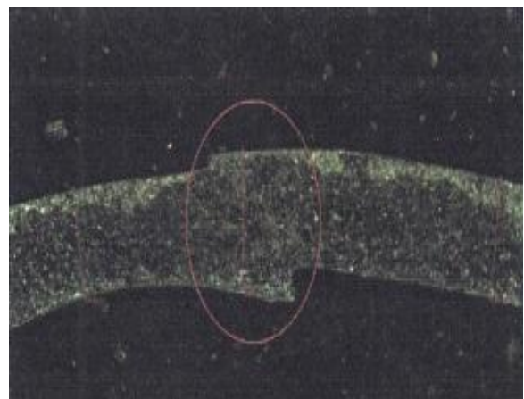
Figure 5 Sheet metal misalignment
