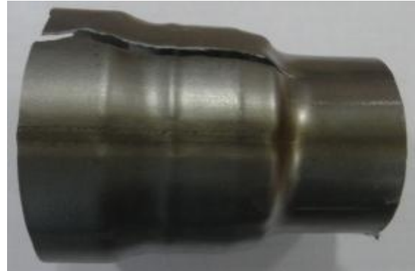
Figure 9 Pipe weld defect
