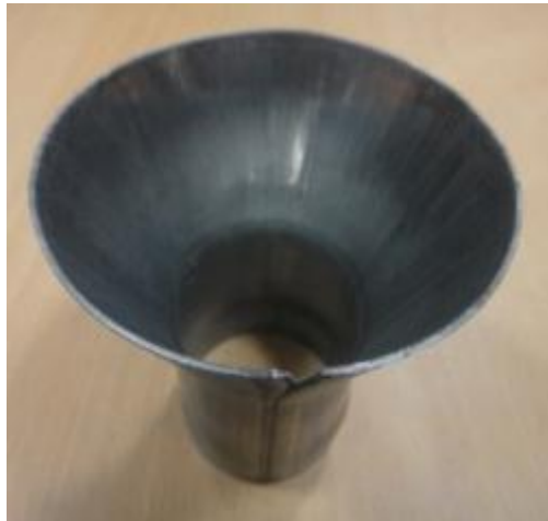
Figure 16 Crack initiated in the weld region
