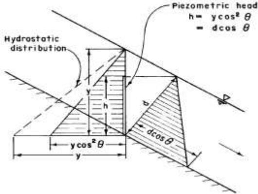
**Fig. 6 Pressure Distribution on Steep slope.**
