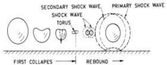
**Fig. 1 Collapse of an individual bubble near a boundary (shown in Falvey [8]).**
