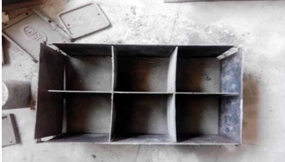
Figure 3.3 Cube Moulds for casting concrete
