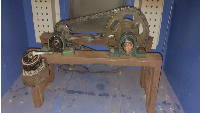
Fig 4 Load Applied over Sprocket and placed in stress freezing oven.
