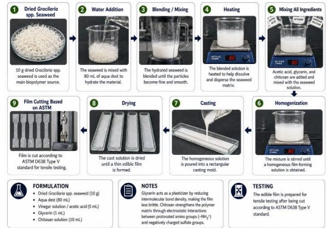
Figure 1. Preparation Process of Gracilaria Spp into Bioplastics up to Testing Stage
