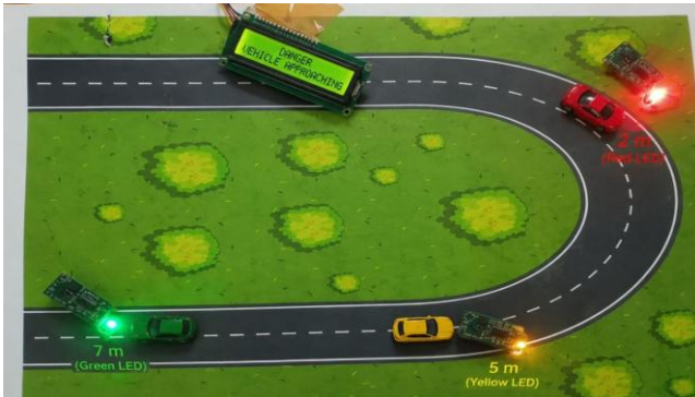
Fig. 5. LCD and LED vehicle-detection status.
