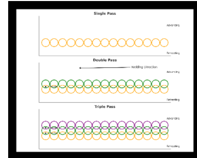
Fig. III. Schematic diagram of the multi-pass friction stir processing process
