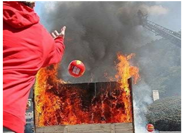
Fig.5 (Embedded ignition chords or fuses (at least two for redundancy) run through the shell.)
