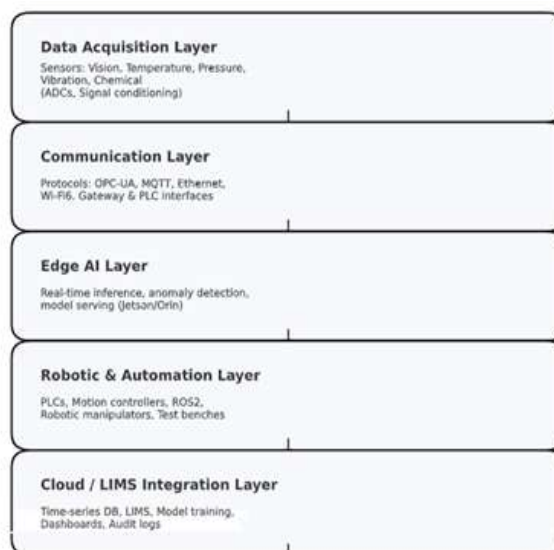
Figure 2 Five layer architecture: autonomous sensor driven laboratory
