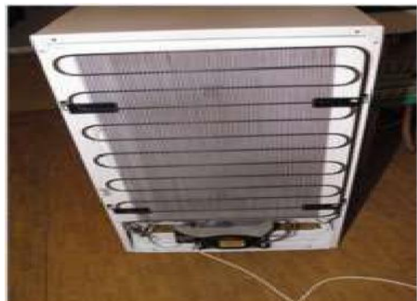
Figure 1: Condensers of refrigerators
