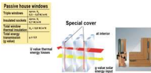
Fig. 22 Triple layered windows that are specific for passive houses
