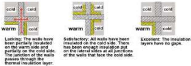
Fig. 14 Thermal bridges at the breaks of horizontal walls
