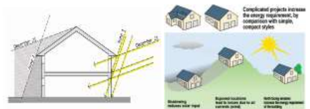
Fig. 2 Aspects regarding orientation, inclination of solar beams and shadowing
