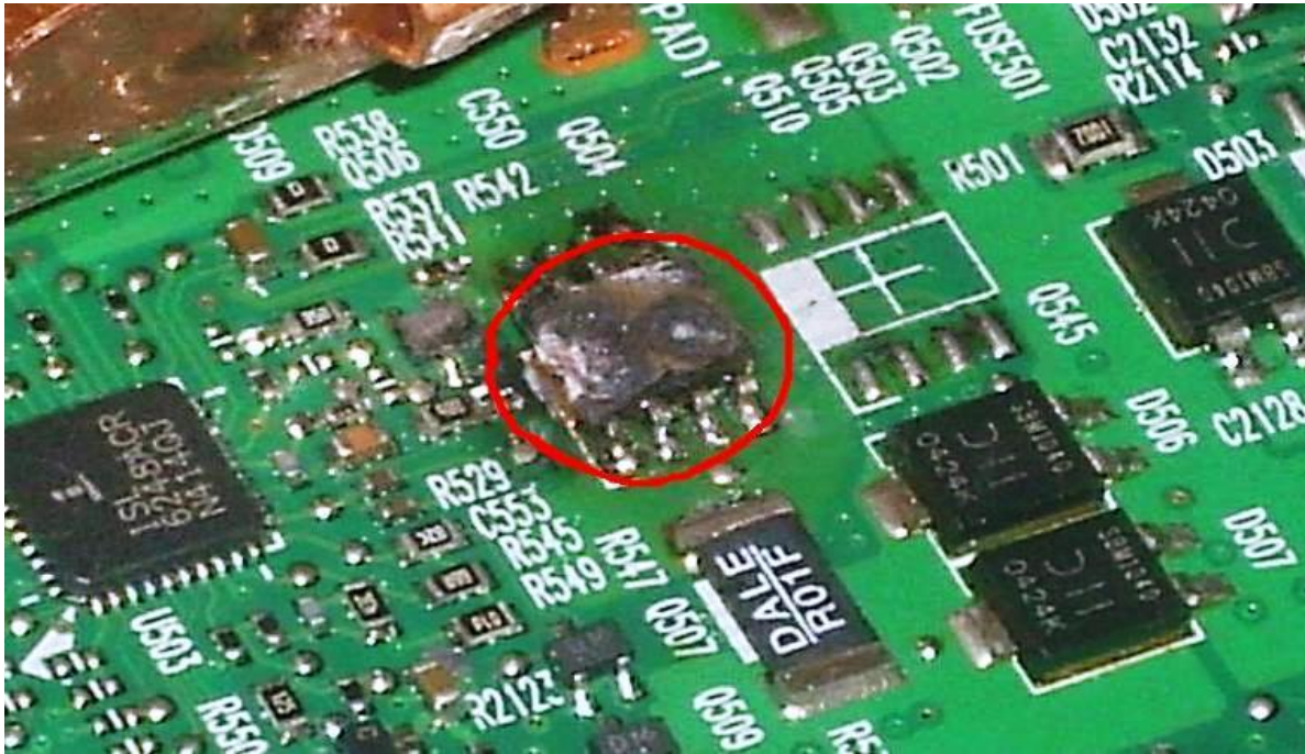
Figure 1 Electronic board with an electronic device damaged by corrosion.
