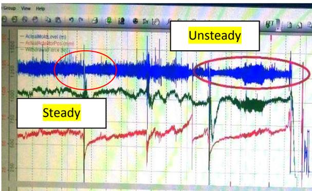
**Fig 7. Mould level fluctuation due to steady and unsteady bulging**
