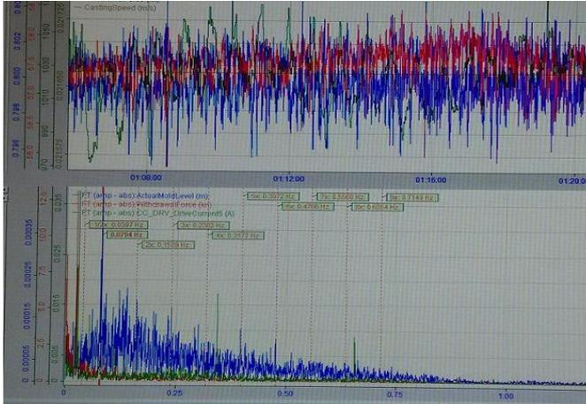
**Fig 9 : Offline FFT to identify segment roll problem**
