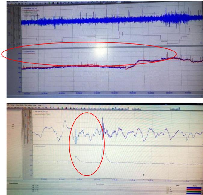
**Fig 3. Mould level peak due to signal Interference**
