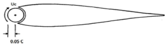
Figure 5. Modified Airfoil NACA 63218 (Chord=0.15m) [2]
