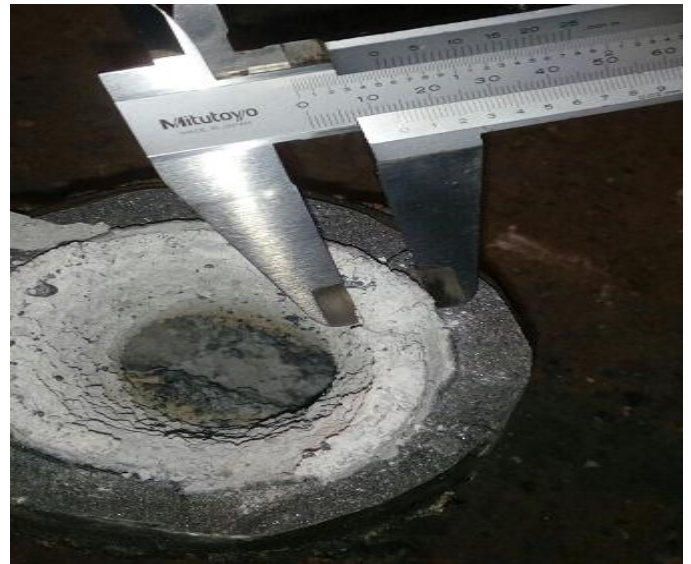
Figure 6: Clogging showing 40% in actual and our model predicted 44.56 %
