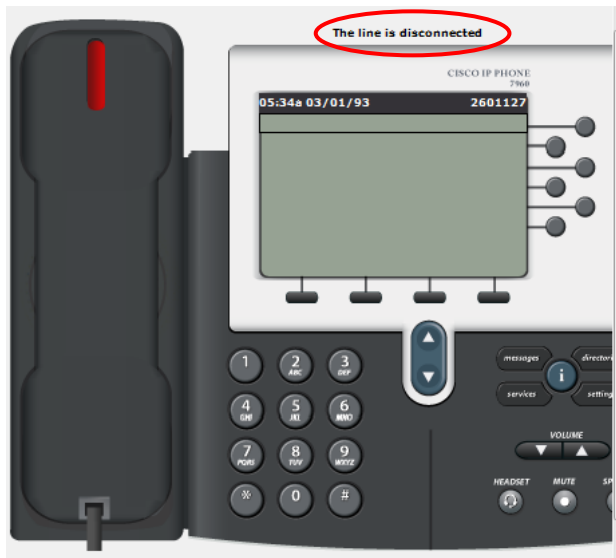
Fig. 6 Callee phone shows the line is disconnected
