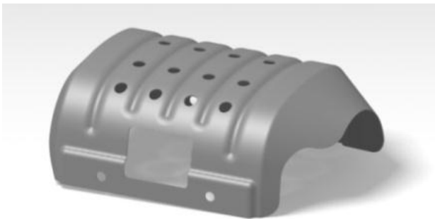
Fig. V Reverse Engineering of Exhaust Heat Shield.
