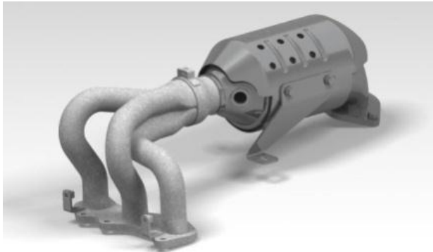
Fig. II Form and Fit checking of Exhaust Hot End Assy.
