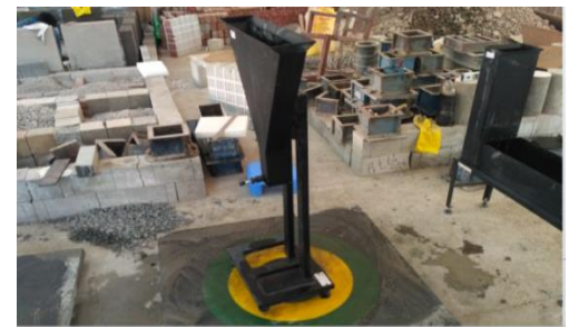
Fig.3.5 set up for V-Funnel test
