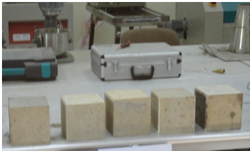
(a) Cubes after curing stage
