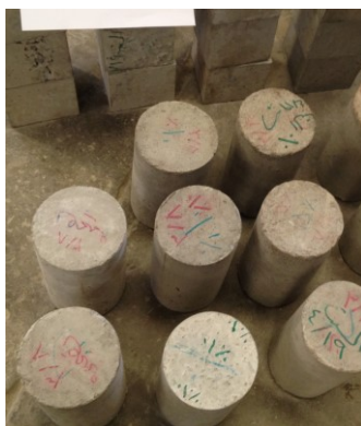
(a) Concrete Cylinder before testing (b) Concrete Brazilian test Figure 3 Cylinder specimen after curing, testing
