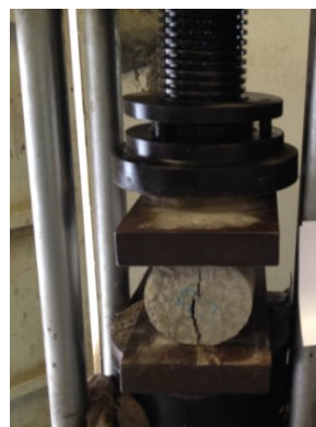
(a) Concrete Cylinder before testing (b) Concrete Brazilian test Figure 3 Cylinder specimen after curing, testing
