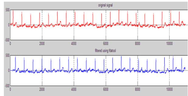
**Figure 3 Kaiser FIR filter output**
