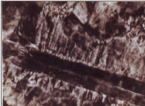
**Figure V Evolution of the matrix crystalline structure in the vicinity of the sized glass fibers**
