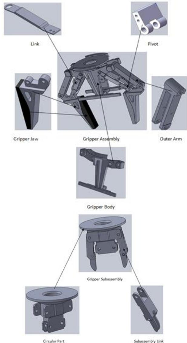
Fig. 4 Gripper Assembly CAD Model
