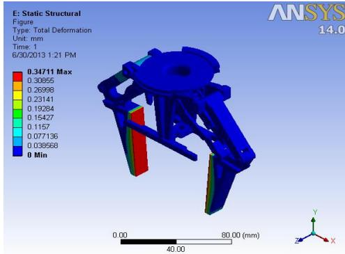
Fig. 9 Gripper Deformation Plot (12kg payload)
