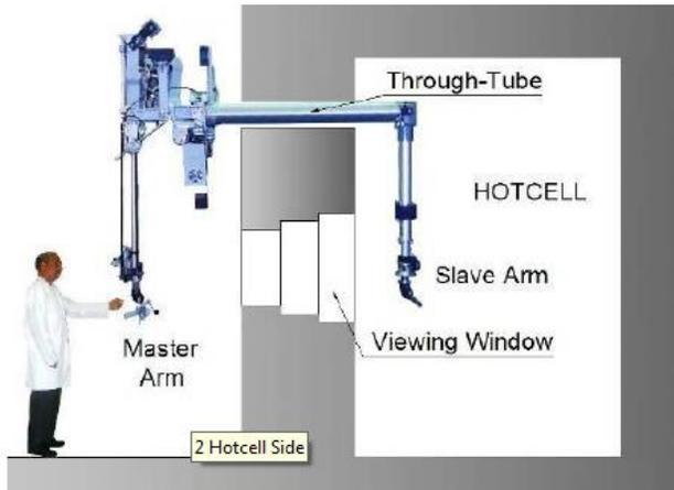
Fig.1 Mechanical Master-slave Manipulator
