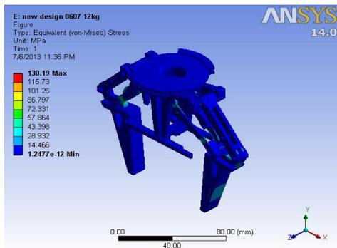
Fig. 15 Modified Gripper Deformation plot (12kg payload)
