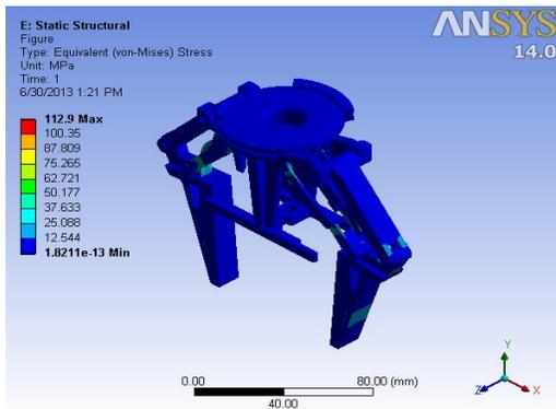
Fig. 10 Gripper Stress Plot (12kg payload)
