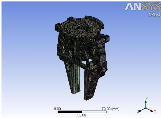
Fig. 4 Gripper Mesh Model
