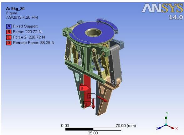
Fig. 5 Gripper Boundary Conditions (9kg payload)
