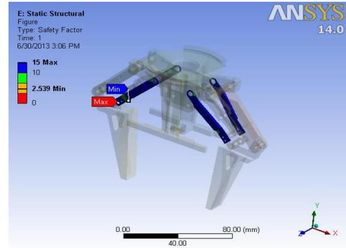
Fig. 11 Link Safety Factor(9kg payload)
