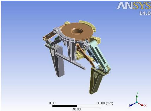
Fig. 13 Modified Gripper Assembly
