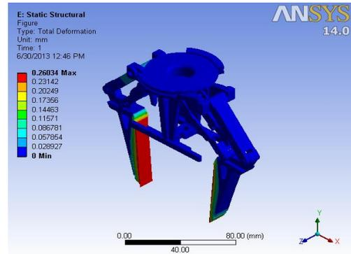
Fig. 6 Gripper Deformation Plot (9kg payload)
