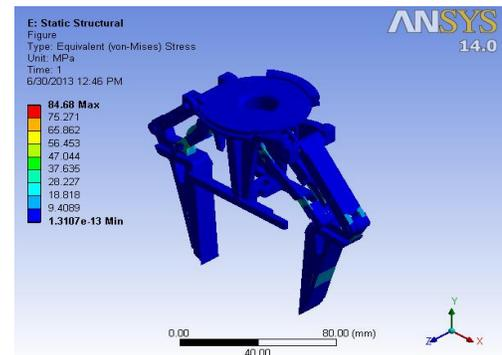
Fig. 6 Gripper Stress Plot (9kg payload)
