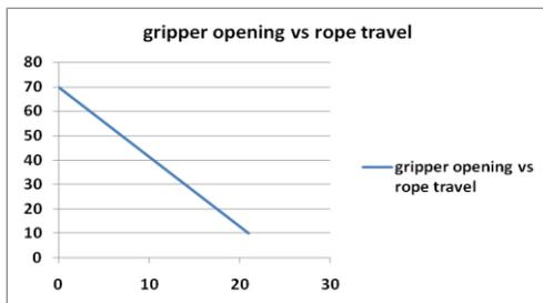
Graph shows variation of rope travel with the gripper opening as the manipulator is operated through pulley wire rope arrangement.
