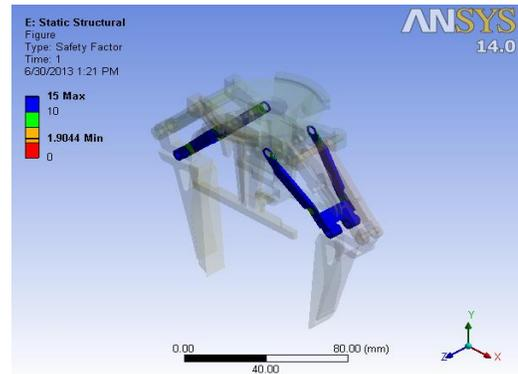
Fig. 12 Link Safety Factor(12kg payload)
