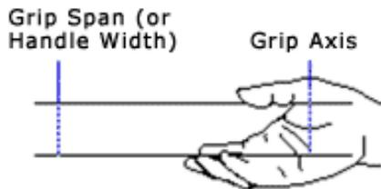
Fig.3 Grip Span for Handle
