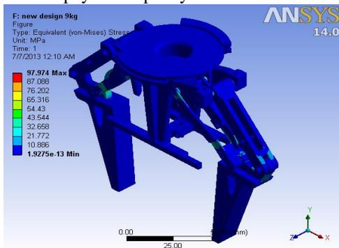
Fig. 14 Modified Gripper Deformation plot (9kg payload)
