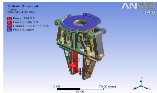
Fig. 8 Gripper Boundary Conditions (9kg payload)
