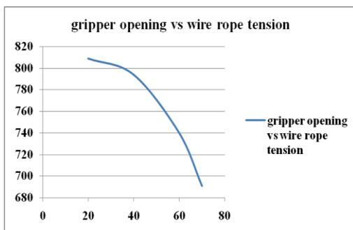
Graph shows variation of tension in wire rope with the gripper jaw opening distance as the manipulator is operated through pulley wire rope arrangement. The tension in wire rope increases with gripper closing. The maximum tension in wire rope is 808 N.
