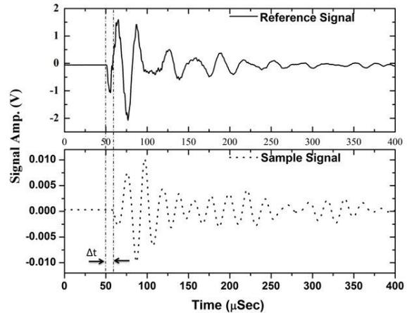
**Fig. 2. Typical example of the reference and the transmitted waveforms used to calculate the transit time  $\Delta t$ .**
