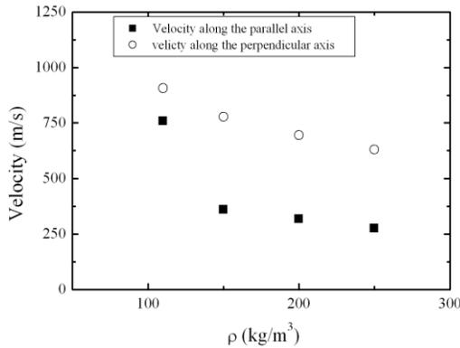
**Fig. 3. Ultrasonic velocity probed along the strain direction (par) and perpendicular to strain direction (per).**
