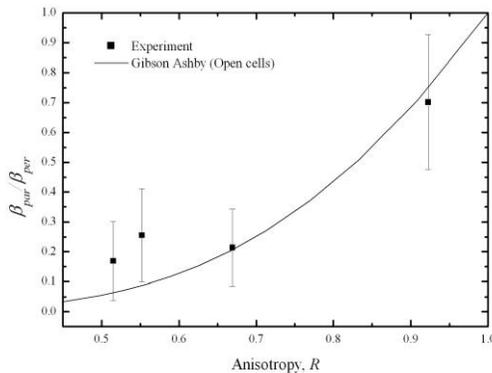
**Fig. 4. The ratio of the longitudinal modulus as a function of cell anisotropy. The solid line represents Gibson and Ashby's open cells model; dotted line represents Gibson and Ashby's closed cells model.**
