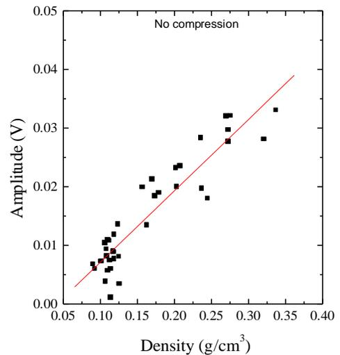
**Fig. 5. The amplitude of the signal taken as an indication of the reduction of the attenuation coefficient as the density of the sample increases.**
