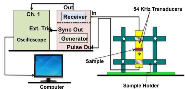
**Fig. 1. Ultrasonic Experimental setup**
