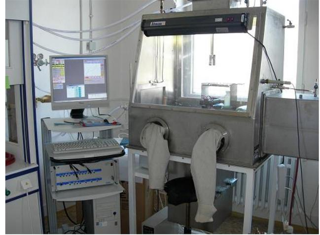
**Fig. 3.** Dry box (Placed in Research Centre Rez)
