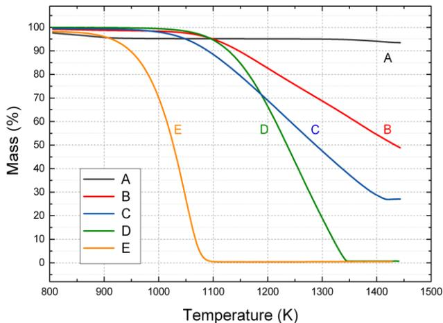
**Fig. 4. TGA analysis material**
