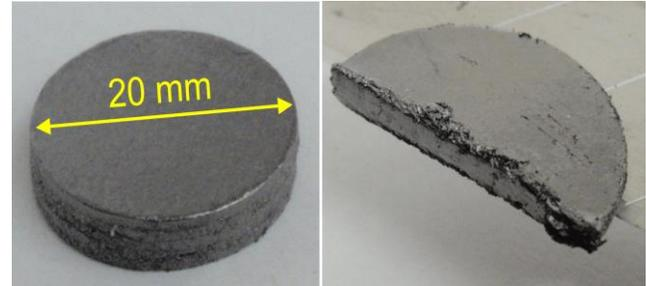
Fig. 1. Graphite sample before testing (left), vertically sample cut (right)
