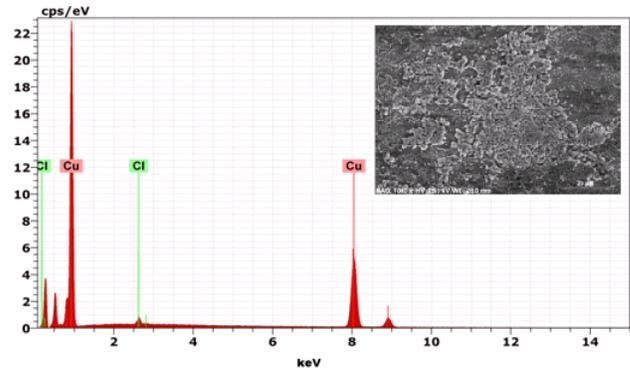
**Figure (8) EDS spectrum of copper electrode potentiostated for 3hrs in 3.5% NaCl. The spectrum was taken from a random spot of surface.**
