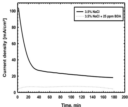
Figure (4) Effect of BDA on the potentiostatic current transients produced by the copper electrode in the presence of 3.5% NaCl only and in the presence of 25ppm BDA
