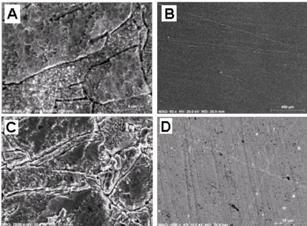
**Figure (7) SEM images of Cu electrode surface at open circuit potential in (a) 3.5% NaCl; (b) 3.5% NaCl+25 ppm BDA; (c) 3.5% NaCl+0.01MHS and (d) 3.5% NaCl+25 ppm BDA+0.01MHS**
