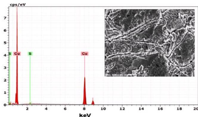
Figure (10) EDS spectrum of copper electrode potentiostated for 3hrs in 3.5% NaCl+25 ppm BDA and 0.01M HS<sup>-</sup>. The spectrum was taken from a spot of white area inside the corroded grain boundary.
