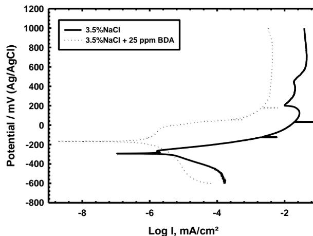
Figure (2) Effect of BDA on the polarization curves of copper in 3.5% NaCl
