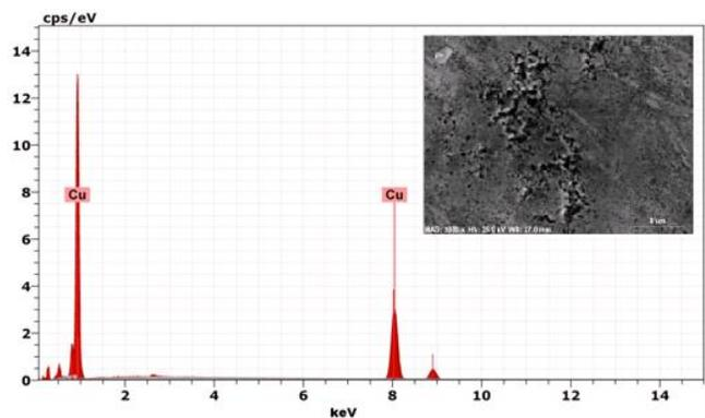
**Figure (9) EDS spectrum of copper electrode potentiostated for 3hrs in 3.5% NaCl+25 ppm BDA. The spectrum was taken from a random spot of surface.**
