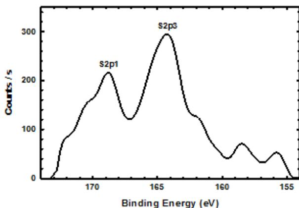
Figure (11) XPS spectrum of the S2p1 and S2p3 signals obtained from the copper electrode in a medium of 3.5% NaCl+25 ppm BDA+0.01M HS<sup>-</sup>
