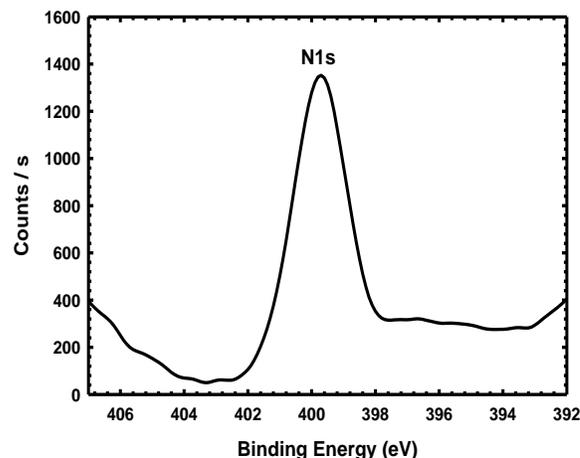
Figure (12) XPS spectrum of the N1s signal obtained from the copper electrode in a medium of 3.5% NaCl+25ppm BDA + 0.01M HS<sup>-</sup>
