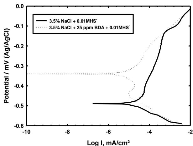
Figure (3): Effect of sulfide ions on the polarization curves of copper in absence and presence of BDA
