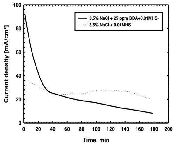
Figure (6) Effect of sulfide ions on the potentiostatic current transients produced by the copper electrode in the presence of 25 ppm BDA
