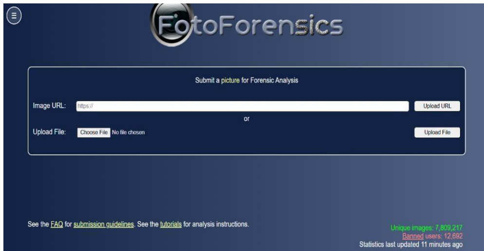
Figure 1 The FotoForensics submission interface utilized for importing image URLs or local files to initiate Error Level Analysis (ELA) and metadata extraction.
