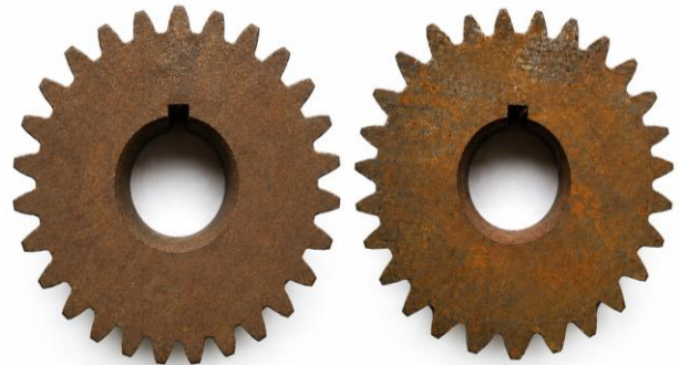
Fig. 1 Symmetric and Asymmetric Spur Gear
