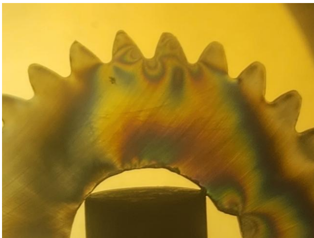
Fig. 7 Isochromatic fringe pattern at tooth root
