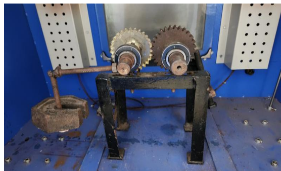
Fig. 4 Load Applied over Spur gear and placed in stress freezing oven.
