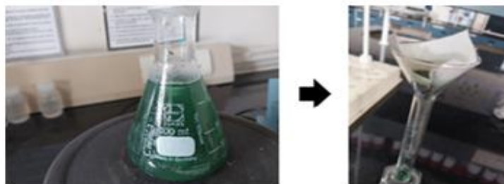
Fig. 4 Preparation of "CuO" NPs by Neem leaves extract.
