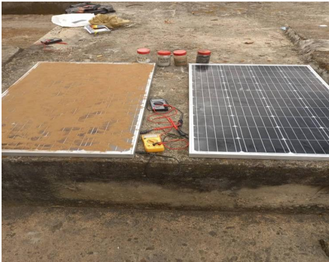
Figure 3. The experimental setup of PV panels, with one sprinkled with environmental dust particles.
