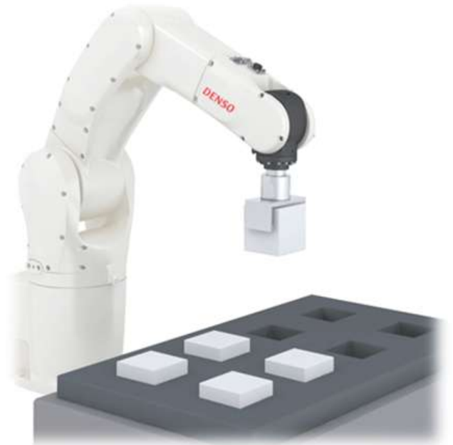
Fig 1. In the above figure the Robot acquire the sensor input. It places the component only if the slot is free.
