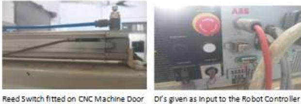
Fig 2 Reed Switches fitted on the CNC Door and DI signal given to Robot
