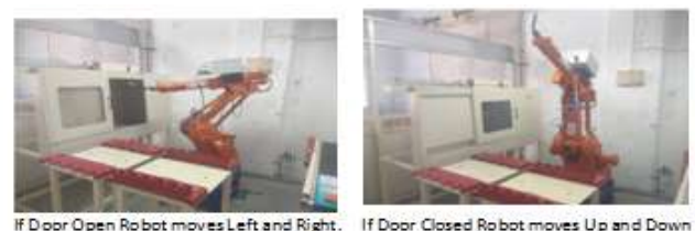
Fig 4. If Door Open Robot moves left and right else moves up and down
