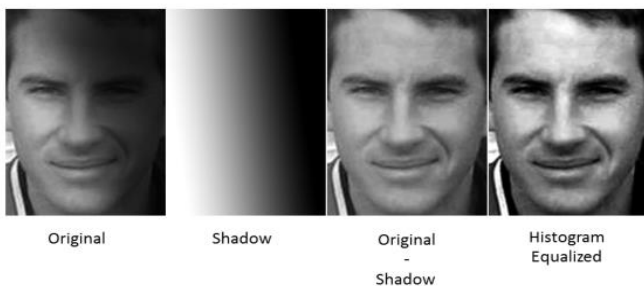
Fig.5. The result of applying a linear filter to the image and as a result, reducing the impact of the shade
