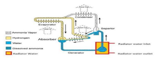
The proposed model is based on three fluid vapour absorption systems. It will contain basic components needed for vapour absorption system as shown in Fig.
